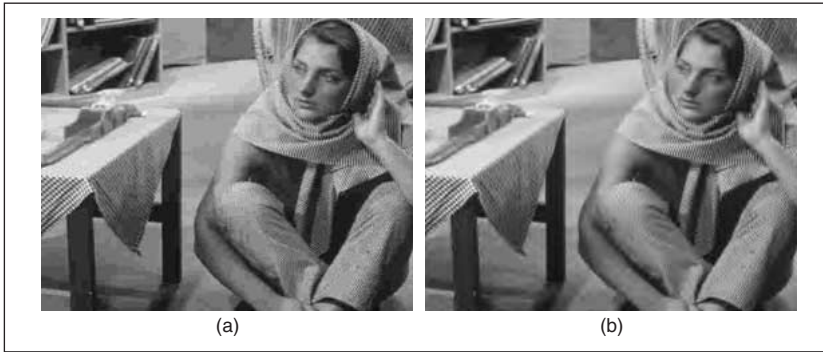
▲ 19. The “Barbara” image coded at 0.3 bits/pixel with JPEG (a) and EZW (b) using a three-level decomposition. The resulting PSNRs for the coded images are 25.1 dB (JPEG) and 26.8 dB (EZW).
