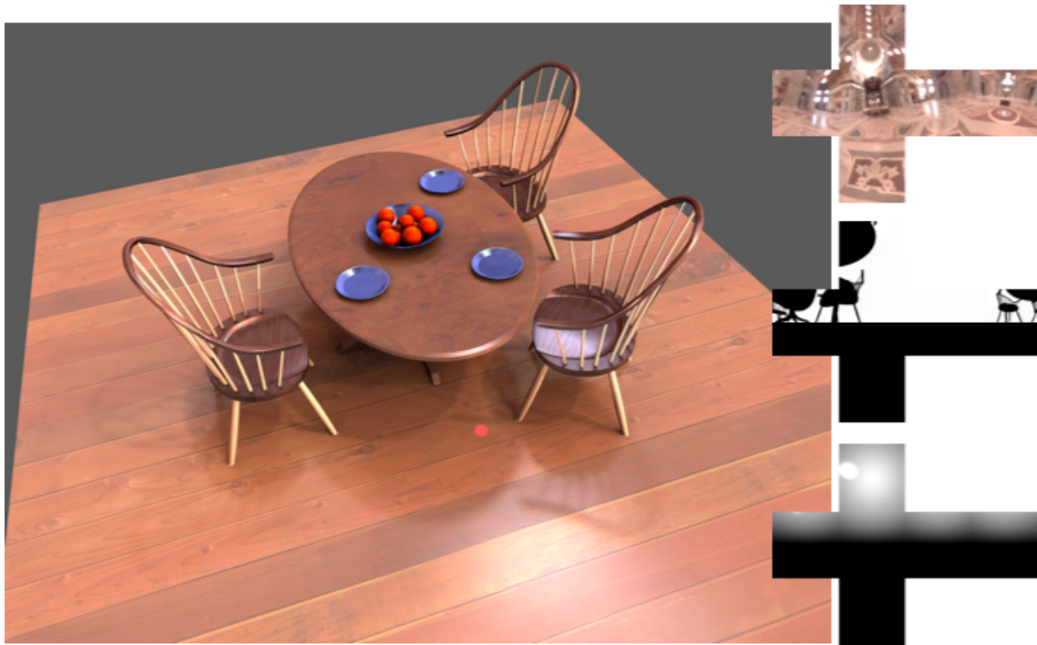
Figure 7: Example image demonstrating the type of output possible using the triple product method. The output scene is rendered on the left. An example lighting cubemap, 4D visibility cubemap, and 4D BRDF cubemap are shown on the right. The pixel for which these cubemaps apply is shown in red in the lefthand image of the scene.
