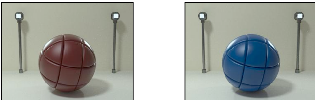
BRDFs for aerosol spray paint
