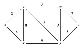
(a) How much flow can we send along the path  $s \to x \to y \to v \to w \to t$ ?
