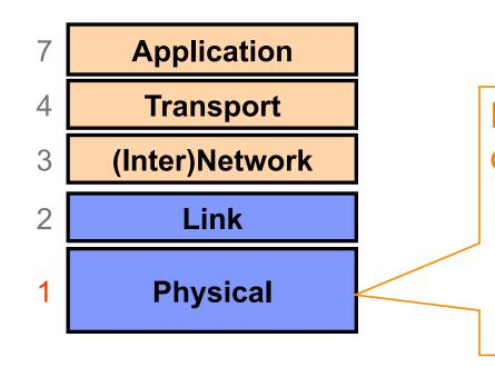
Encoding bits to send them over a <u>single</u> **physical link** e.g. patterns of *voltage levels / photon intensities / RF modulation*
