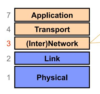
Bridges multiple "subnets" to provide *end-to-end* internet connectivity between nodes • Provides <u>global</u> <u>addressing</u>
