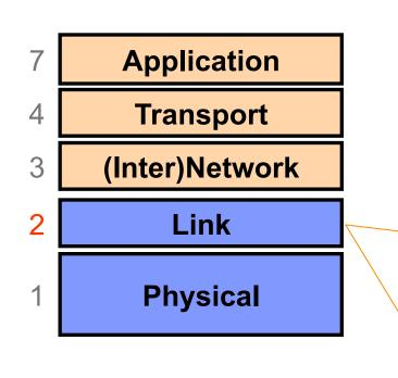
Framing and transmission of a collection of bits into individual messages sent across a single "subnetwork" (one physical technology)
